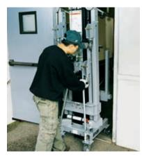
The compact stowed position makes the Super Tower lift easy to move through doors and load on trucks with no bulky base to get in the way. Stowed dimensions are 22 in (56 cm) by 25.25 in (64 cm).
